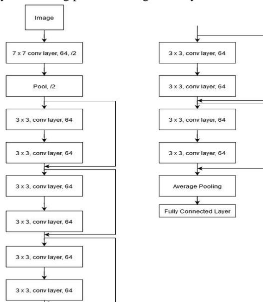
Fig. 1. Residual Neural Network Architecture
