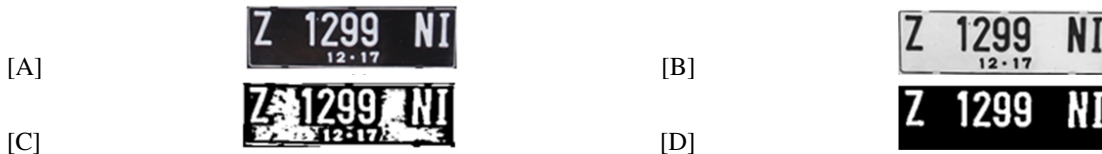
Fig. 3. (A) input (B)resized and converted image into grayscale (C)resized and converted image into grayscale (D) result after labelling and analysing process
